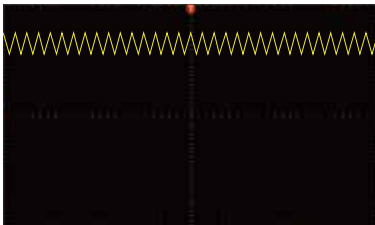
DC+AC Vdc=50V, triangle ripple Vac=5V, frequency 150Hz
